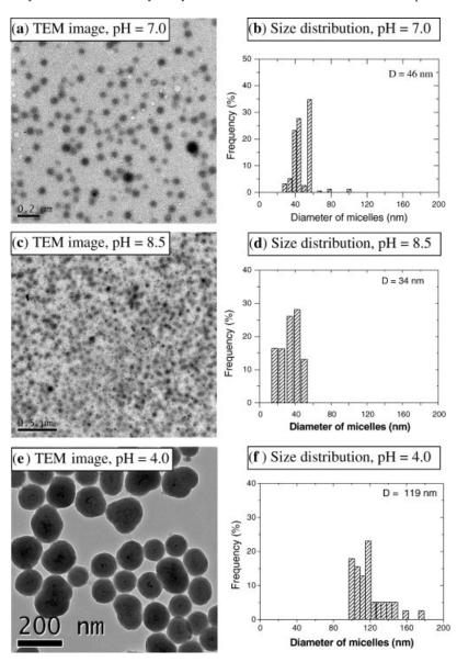
**Figure 3.** TEM images (a, c and e) and corresponding size distributions (b, d and f) of the self-assembled micelles in aqueous solution at pH = 7.0, 8.5, and 4.0, respectively, from the amphiphilic pentablock copolymer PDMAEMA-b-PTFEMA-b-PDMAEMA.  $M_{n,GPC}$  = 59170 g/mol, PDI = 1.43.
